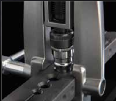
Push down the yoke and with fewer rotations, you get a precise flare or swage.
